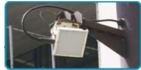
ITS Spot (roadside antenna)
