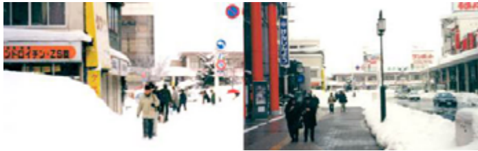
WITHOUT ROAD HEATING WITH ROAD HEATING FIGURE 10 - EFFECT OF ROAD HEATING SYSTEM
