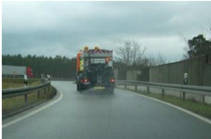
COMBI-SPREADER WHICH CAN SPREAD BOTH: PRE-WETTED SALT OR BRINE ONLY
