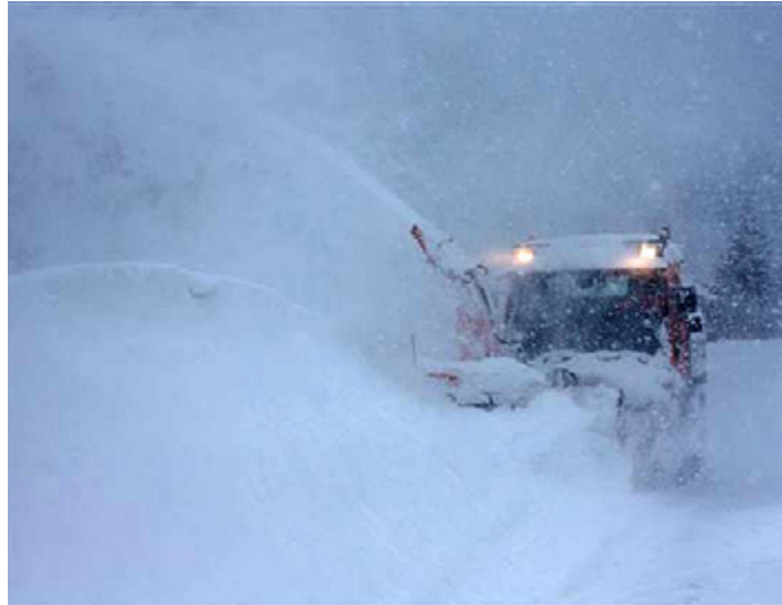
FIGURE 3 – SNOW CUTTER BLOWER IN THE AREA OF LILIENFELD (LOWER AUSTRIA)
