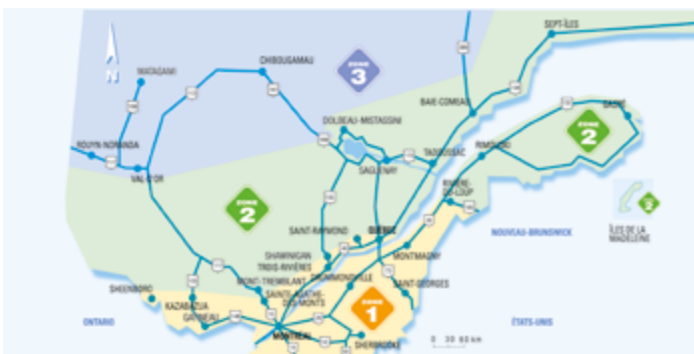
FIGURE 3 - LOAD RESTRICTION AREAS
