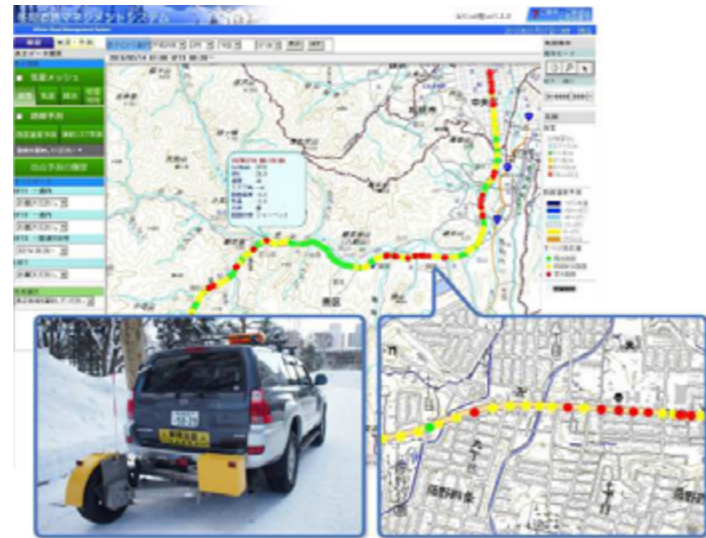
TOP: WINTER ROAD FRICTION PROVISION SYSTEM DISPLAY LEFT BOTTOM: TEST VEHICLE WITH A CONTINUOUS SKID-RESISTANCE MEASUREMENT DEVICE. RIGHT BOTTOM: ENLARGED ROUTE MAP SHOWING MEASURED SKID RESISTANCE
