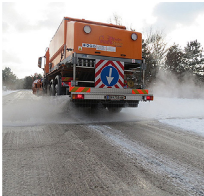
FIGURE 5 – TRUCK “FIRESTORM” WITH BRINE SPRAYING DEVICE
