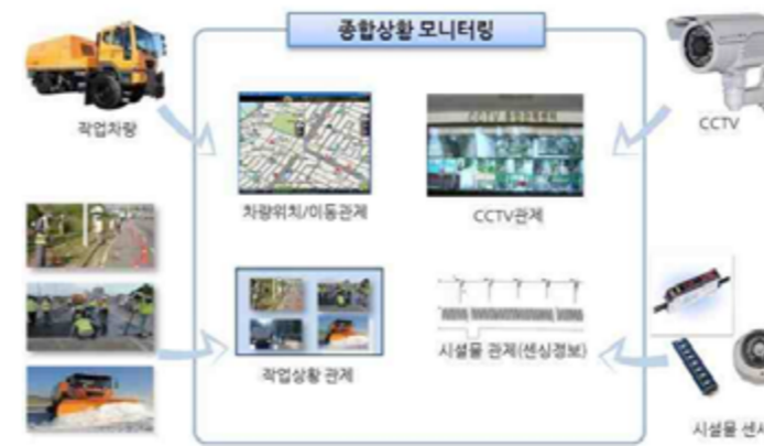
FIGURE 6- ROAD SURFACE MONITORING SYSTEM
