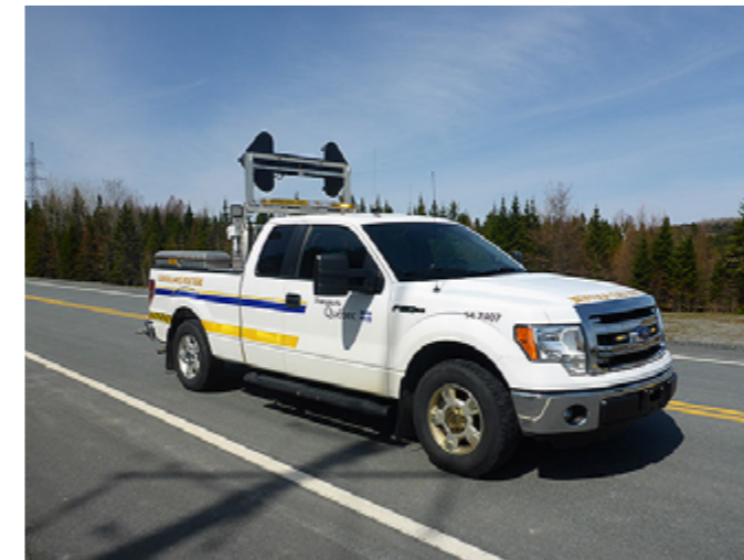
FIGURE 6 – MOBILE ROAD WEATHER STATION
