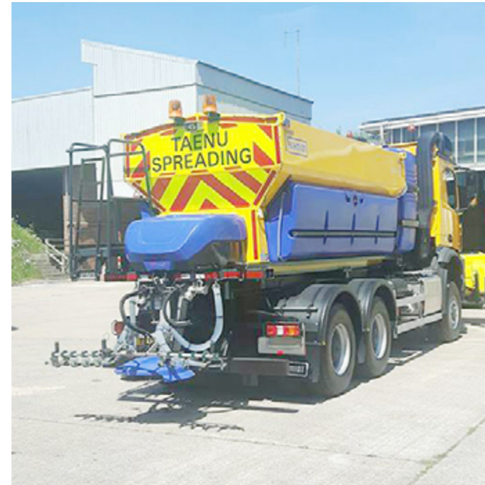
NEW WELSH GOVERNMENT COMBI (SOLID / LIQUID) SPREADER WITH VIEW OF SPRAY BAR AND SPINNER ASSEMBLY
