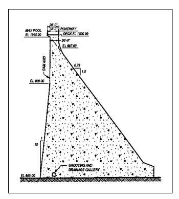
Figure 2-2. Nonoverflow section
