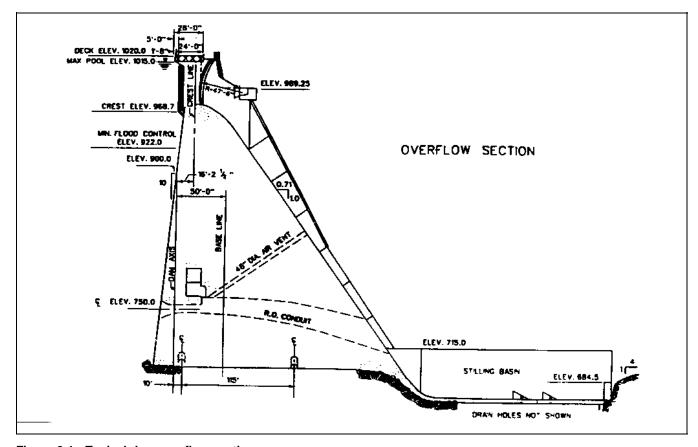
Figure 2-1. Typical dam overflow section
