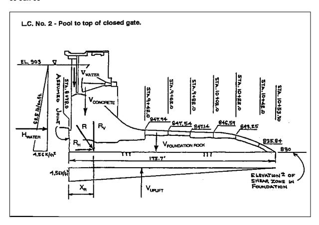
Figure 8-2. Free body diagram,  $R_y$  = resultant of vertical forces,  $R_H$  = resultant of horizontal forces, and  $X_R$  = distance from heel to resultant location on sliding plane
