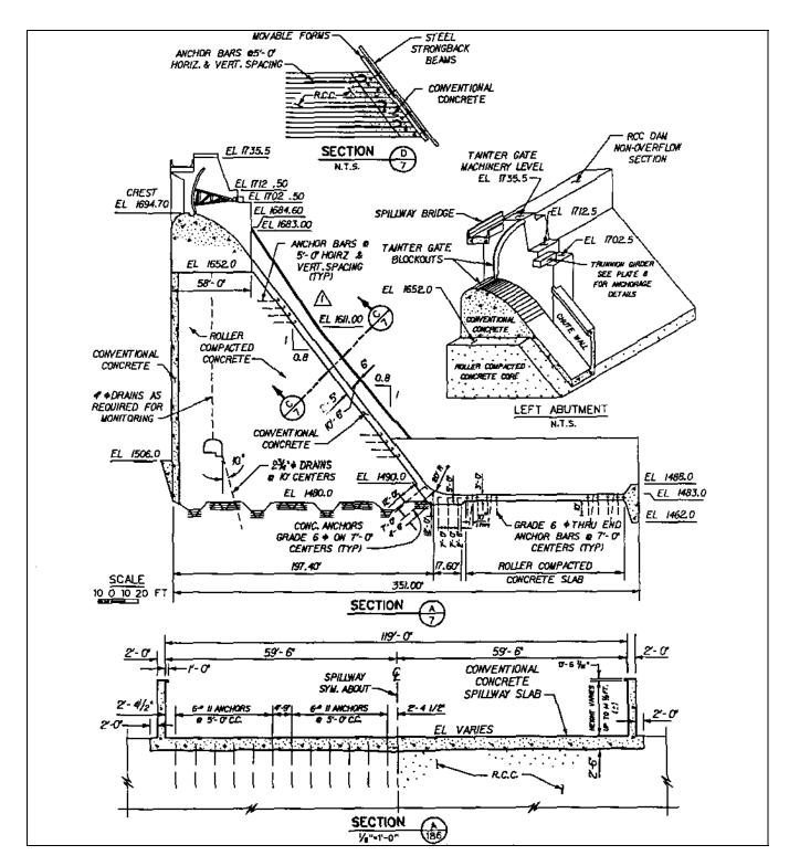
Figure 9-6. RCC spillway details
