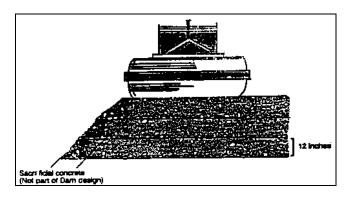
Figure 9-3. Compaction of RCC at downstream face
