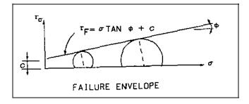
Figure 4-3. Failure envelope
