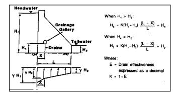
Figure 3-2. Uplift distribution with drainage gallery
