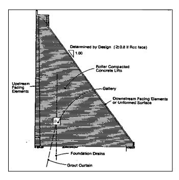
Figure 9-1. Typical RCC dam section
