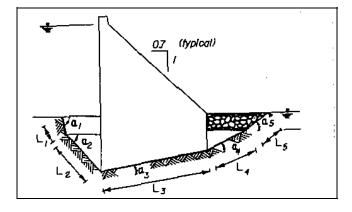
Figure 4-4. Geometry of structure foundation system
