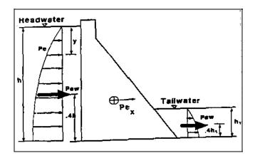
Figure 3-10. Seismically loaded gravity dam, nonoverflow monolith
