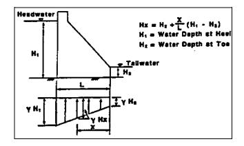
Figure 3-1. Uplift distribution without foundation drainage
