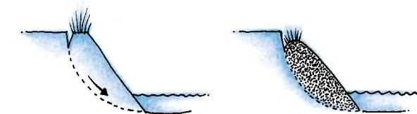
(c) Deep-seated rotational failure slope failure → toe failure → base failure
