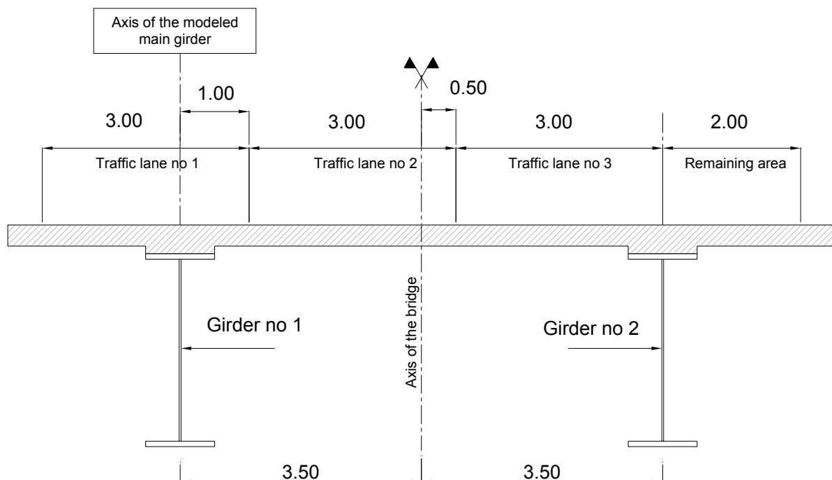
Figure 5.2: Positioning the traffic lanes for calculating the girder no 1 in longitudinal global bending
