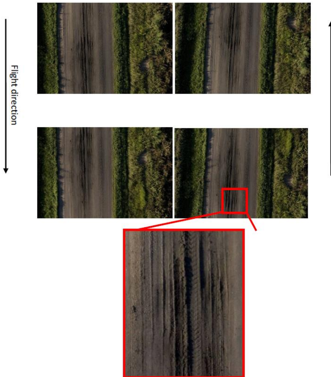
Figure 4.1.5.5. Example of road images acquired by UAV over a road segment. The segment was captured 4 times in a single mission. The flight directions are indicated by arrow lines. The bottom image shows the fine details of road feature (ruts) in original resolution.
