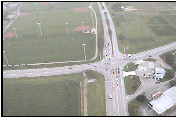
Figure 4.3.2.2, An example of circling a facility with the UAS, (A) looking west at the intersection of the Kenny Rd and Lane Ave, (B) a second view looking east at the same intersection illustrating the changing perspective when circling a facility. Note that the queue lengths and turning movements are visible in these images.
