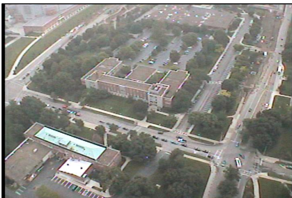
Figure 4.3.2.2, An example of circling a facility with the UAS, (A) looking west at the intersection of the Kenny Rd and Lane Ave, (B) a second view looking east at the same intersection illustrating the changing perspective when circling a facility. Note that the queue lengths and turning movements are visible in these images.
