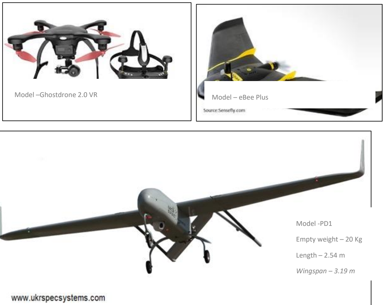
Figure 3.1: Top left is a multi-rotor Ghostdrone 2.0. Top right is a fixed wing eBee Plus UAS. Bottom is fixed wing PD-1 UAS.
