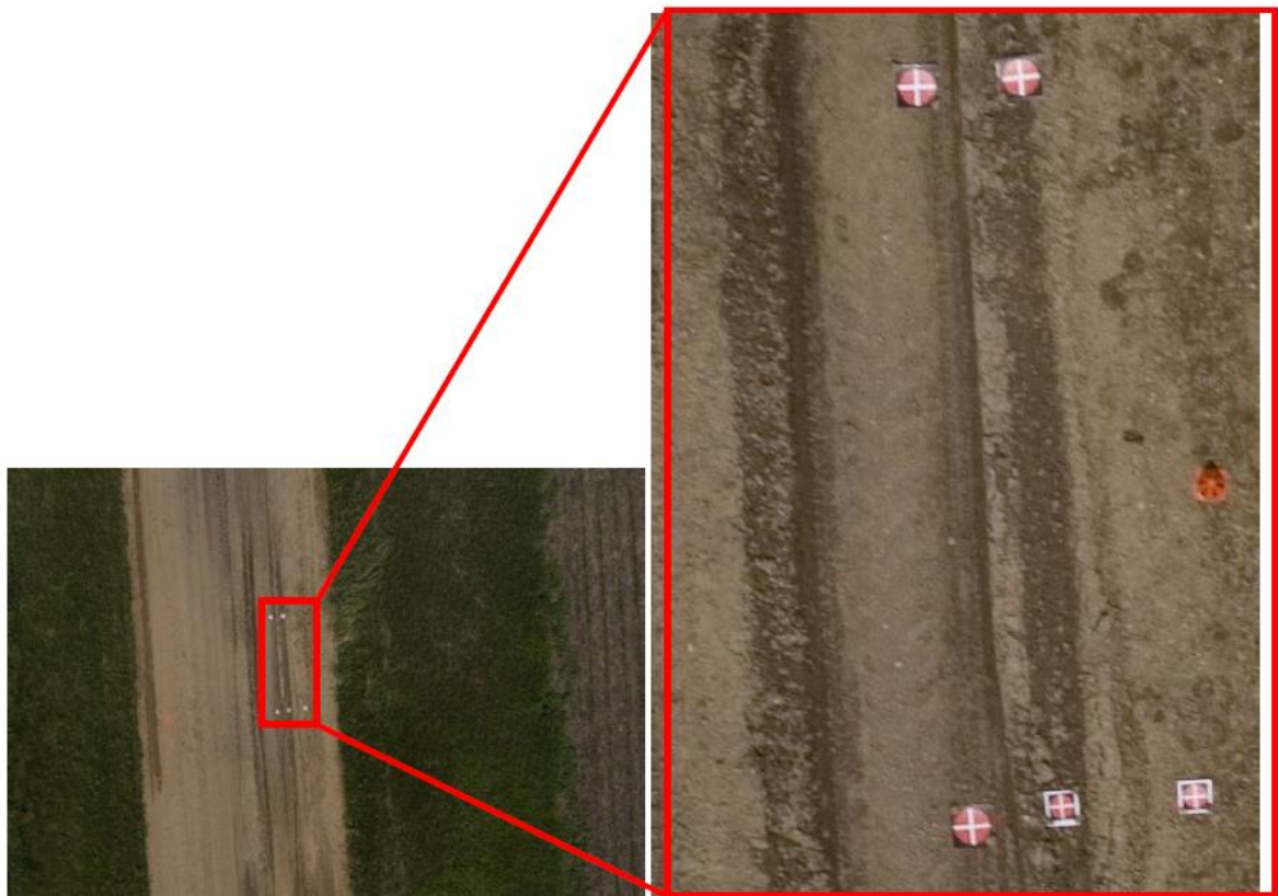
Figure 4.1.5.7 Road image acquired by UAV showing severe ruts. Note the marks are designed for ground measurements and for relating ground measurements with image measurements.
