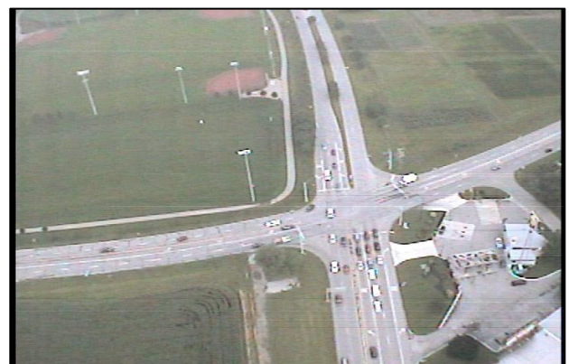
Figure 4.3.2.2, An example of circling a facility with the UAS, (A) looking west at the intersection of the Kenny Rd and Lane Ave, (B) a second view looking east at the same intersection illustrating the changing perspective when circling a facility. Note that the queue lengths and turning movements are visible in these images.
