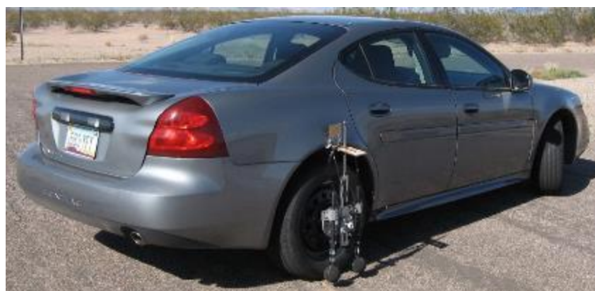
Figure 25. OBSI measurement system in practice. [95].
