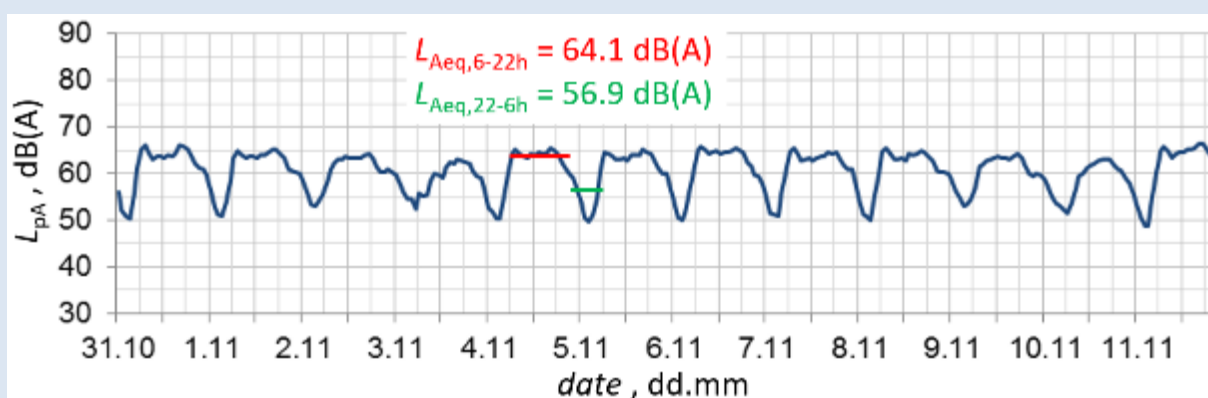
Figure 32: Environmental noise monitoring - road traffic noise measurement at a receiver point.
