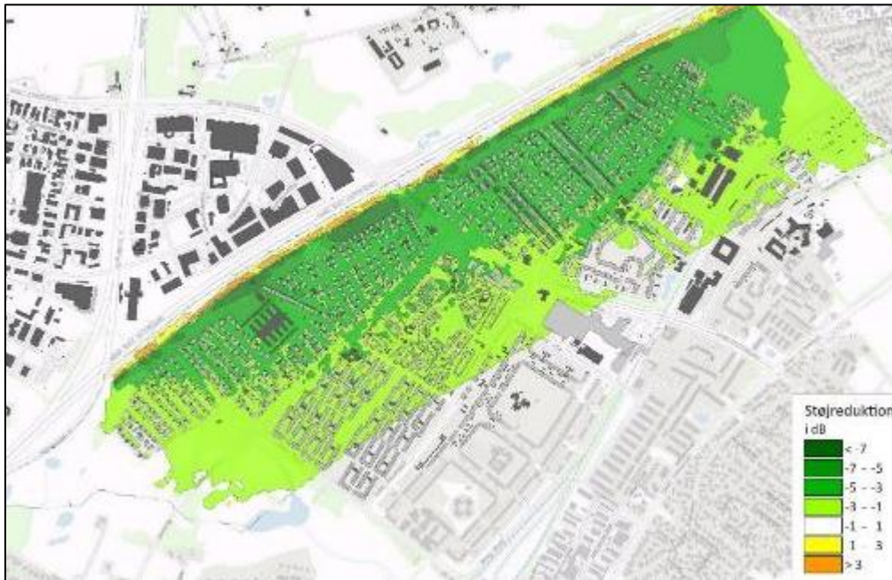
Figure 40: Differential noise maps showing the noise reduction due to increasing a bank of earth from the height of 6 m to 12 m. The map shows the predicted noise reduction.
