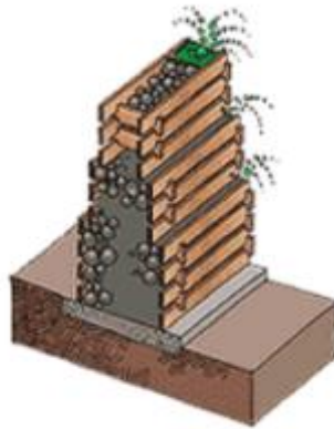
Figure 83: Bio barrier with wooden structure. [165]
