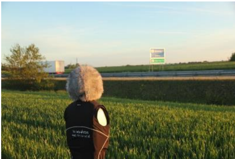
Figure 42: Recording vehicle passing by using HATS. (Source: Per Finne, DELTA Acoustics)
