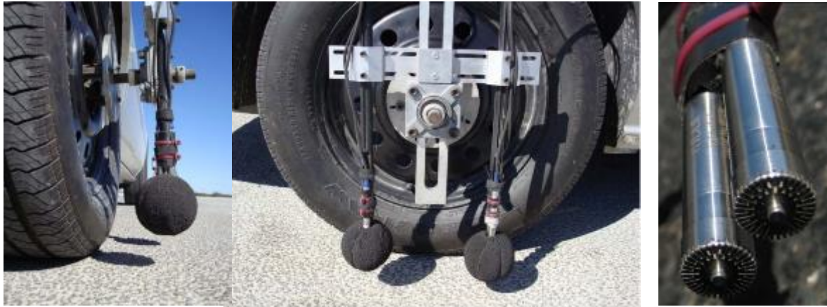
26a) and 26b) Close-up view of the positioning of the sound intensity probes, probes protected by means of wind shields
