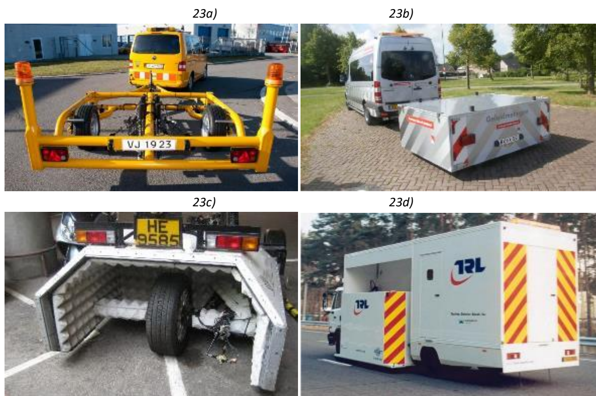
Figure 23. CPX measuring vehicles. a) open trailer with two test tyres operated by the Danish Road Directorate, Denmark (DRD). Source: M+P Consultants. b) closed trailer with two test tyres operated by Province of Noord-Brabant, The Netherlands. Source: M+P Consultants. c) open trailer with one test tyre operated by Tin Shun Consultants, Hong Kong, Source: www.hktscl.com.hk d) self-powered vehicle with one test tyre operated by the Transport Research Laboratory TRL, United Kingdom. [96].
