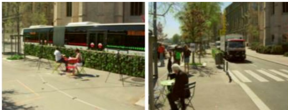
Figure 80: Questionnaire respondents and acoustic measurement equipment behind the low height barrier (left) and at the side of the barrier right). [164]
