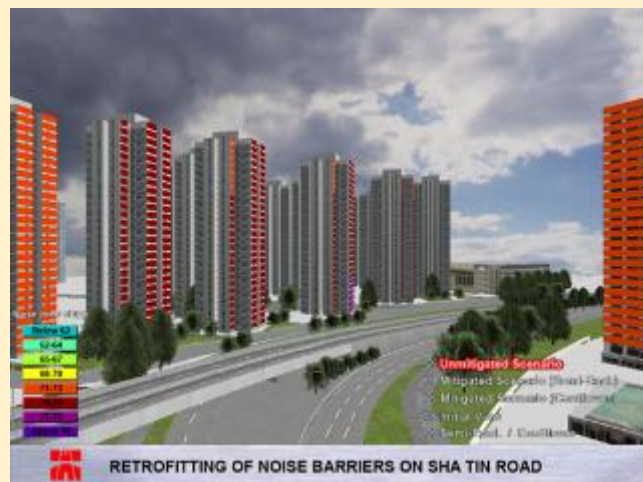
3D model of Sha Tin Road shows noise levels at different heights
