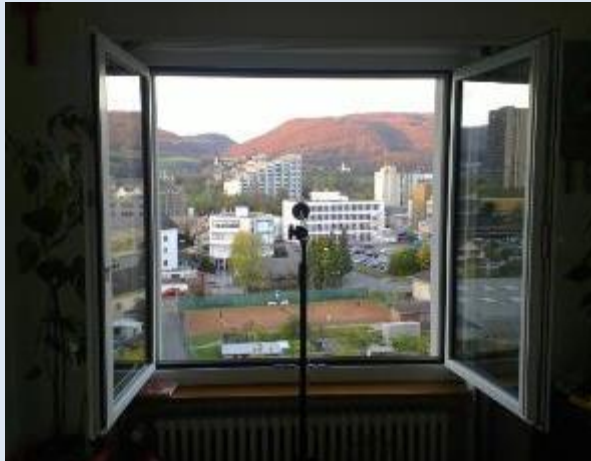
Figure 30: Road traffic noise impact measurement. a) free field measurement; b) quasi-free field (substitutional microphone position); c) open window microphone positioning seen from inside; d) boundary layer positioning. (Source: Müller-BBM).
