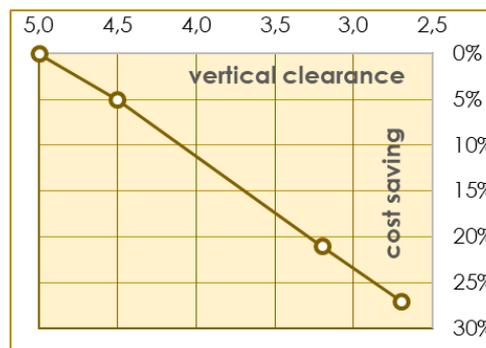
Figure 3 - Construction costs saving versus vertical clearance
