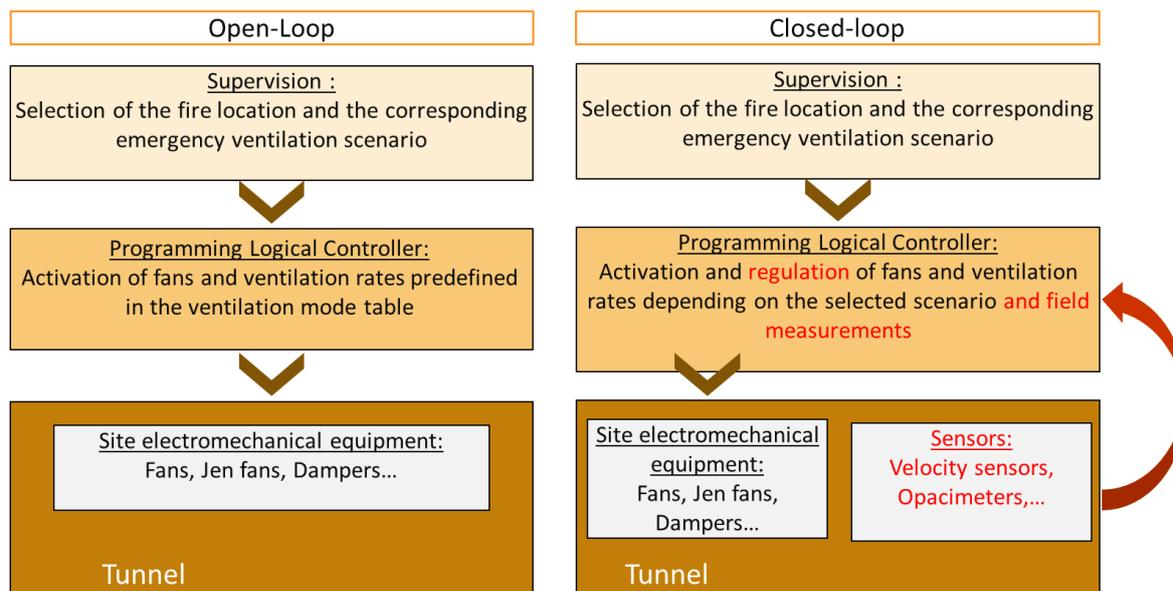
Figure 7 - Illustration of open-loop versus closed-loop control of the ventilation system
