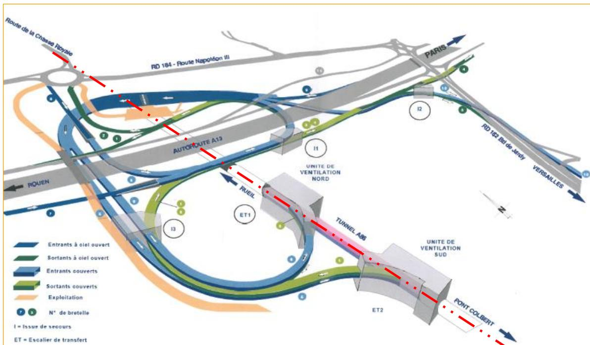
Figure 2 - Example of a complex underground infrastructure -underground interchange between Duplex A 86 and motorway A13 in the Region Ile-de-France. (See monograph 2-8)
