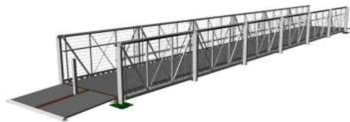
Figure 5.12: Modular footbridge with variable span 3.0-18.0 m.
