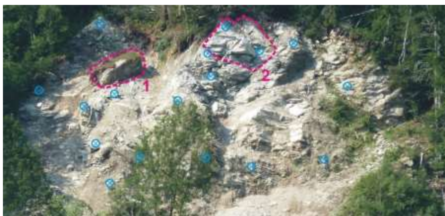
1: large rock boulder blasted on 2012/07/24, 2: rock failure occurred on 2012/07/26, Blue circles: position of geodetic targets
