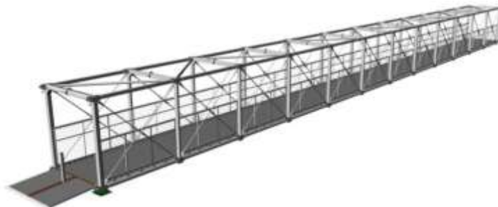
Figure 5.13: Modular footbridge with variable span 3.0-36.0 m.
